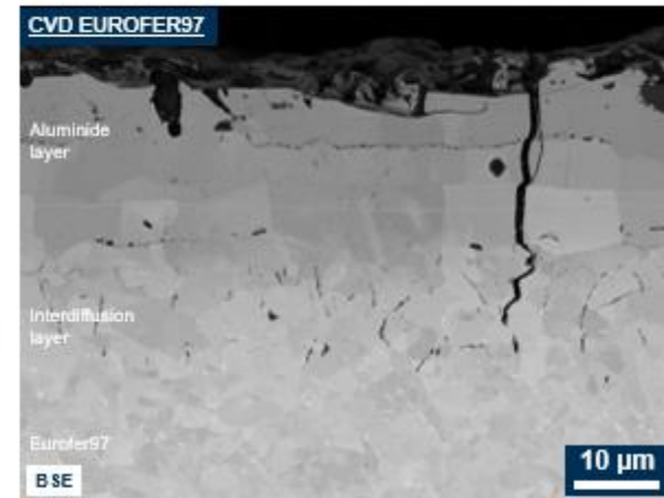
Fig. 10 ↑: Representative cross-section of the cracked EUROFER97 coated with the CVD Al-base coating after engineering straining at \approx 1\% .
